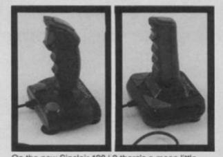
On the new Sinclair 128+2 there's a mean little message above the newly added joystick ports. It says "Use only Sinclair SJS1 joysticks". Sinclair/ Amstrad have been very canny in reconfiguring the wires in their joystick ports so your average bogstandard Kempston won't work. Not to be upset by this, Cheetah has added an extra plug to its new Sticks of Joy, specially to fit the +2! And if you don't want to bin your existing joysticks, Cheetah's also brought out an adaptor that'll make them fit.
